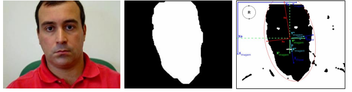
Fig. 2. The image face skin color detection with the face detected area and the fitted ellipse.
